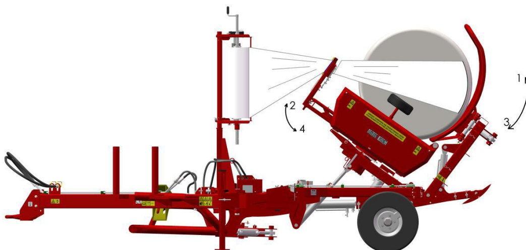
Fig. 22. Unloading of a bale to the bale on end kit's cradle. The figures next to arrows show the correct order of movements of working units during unloading.
